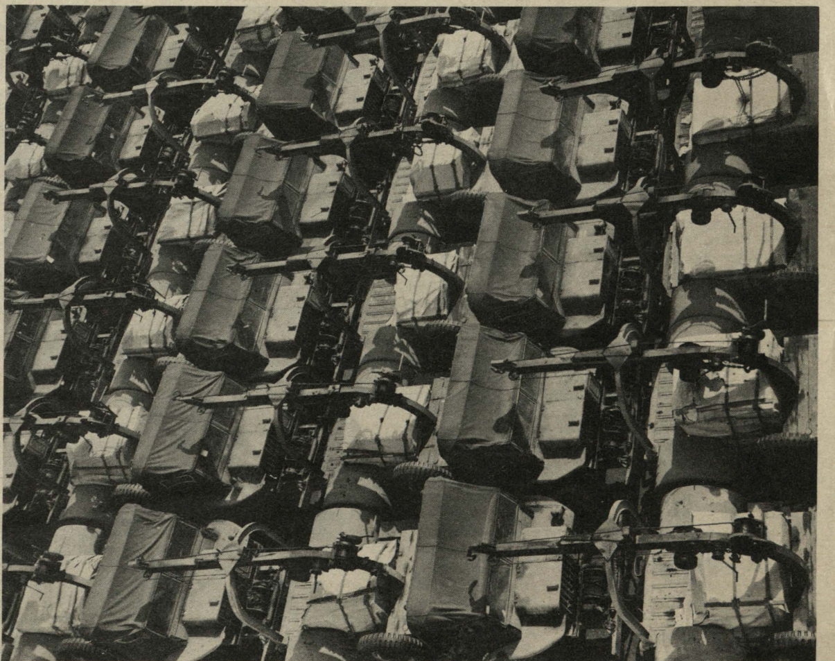
War Reserve Storage A portion of about 100 navy bomb loaders that are being put aboard LST's of the 19th fleet at the Swan Island dock make an interesting pattern picture from above. Unused, these trucks are preserved in accordance with the Bureau of Shipping manual for war reserve storage.
