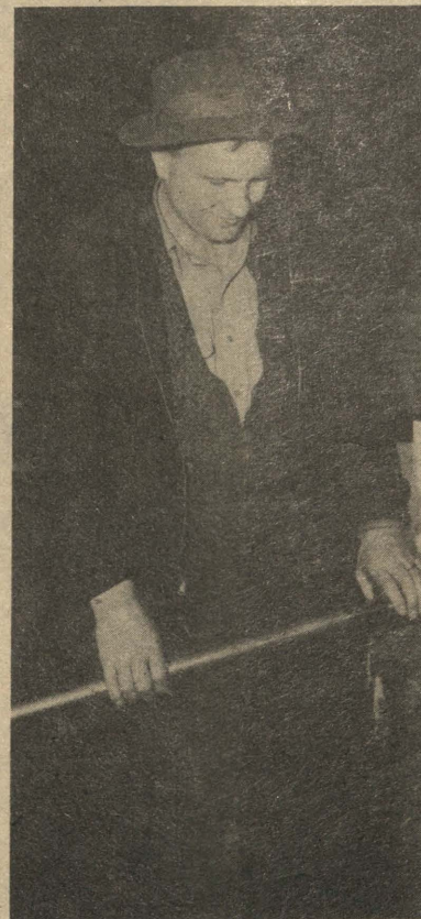
Al Jensen, shipwright supervisor in charge of launching crews, stands by one of the massive hand-operated jacks which are located on each side of the launching fore-poppet in case a ship's hull should require "a little coaxing" to start down the ways. The jacks have been needed only "a couple of times," Jensen said.
